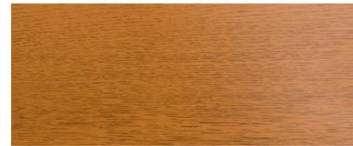
40 µm thick polyester paint with Z275 zinc layer or ZM120 zinc-magnesium layer. It is characterised by its wood structure and adequate protection against corrosion and UV radiation. This combination allows outdoor use, especially where high weather resistance and high aesthetics are required.
